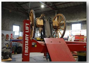
Note the photo above of Dayna Barscello, Assistant Curator, working above on a vehicle lift. Dayna decided to put the carriage on a hoist with the trail to the ground. She did this to make her job more effective. This way the conservation epoxy soaked deep into the cracks of the wood. This in turn helped consolidate any accident damage. Well done Dayna! We now have five wooden wheeled cannons, including the damaged 9 pounder, in our Heritage Gallery.
