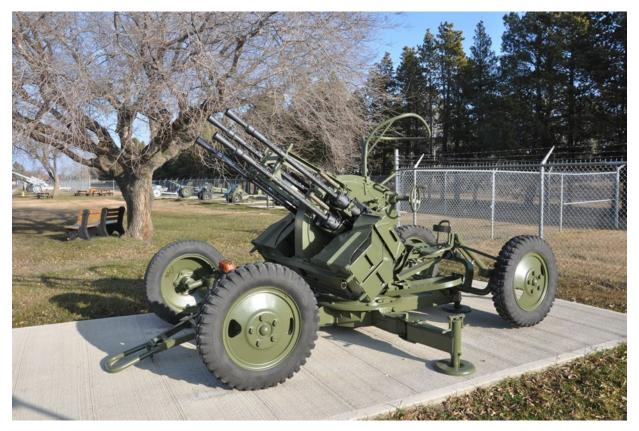
The ZPU is a family of Russian designed anti-aircraft machine guns used by over fifty countries, not including Canada. There are four main variants: the quadruple-barreled ZPU-4 (which The RCA Museum exhibits), two double-barreled (ZPU-2 and ZU-2) and a single barreled version the ZPU-1. Each barrel is air cooled with a maximum firing rate of 600 rounds per minute. The ZPU-4 employs a four-wheeled carriage and is still currently in use around the world.
