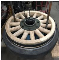
Our wheelwright certainly had a big challenge on his hands. He needed to build a jig for the wooden fellows and a specialised press. Note the picture to the right. He also determined that our original steel rims were heavily corroded and required some restoration. To accomplish the task of pressing the wooden fellows into the steel rim, he built a press out of two 50 ton jacks. The actual pressing required approximately 60 tons of force. Note the completed wheel
