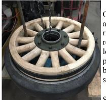
Our wheelwright certainly had a big challenge on his hands. He needed to build a jig for the wooden fellows and a specialised press. Note the picture to the right. He also determined that our original steel rims were heavily corroded and required some restoration. To accomplish the task of pressing the wooden fellows into the steel rim, he built a press out of two 50 ton jacks. The actual pressing required approximately 60 tons of force. Note the completed wheel
