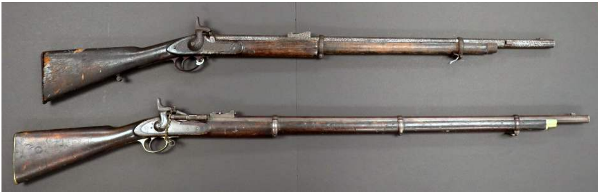
Top: Pattern 1853 Enfield; bottom: converted Pattern 1853 Enfield (Snider-Enfield Rifle Mark I)
